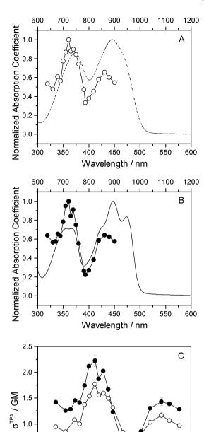
Fig. 3 Experimental data. (A) Two-photon (open circles) and one-photon (dashed line) absorption spectra of FMN. (B) Two-photon (filled circles) and one-photon (solid line) absorption spectra of miniSOG. (C) The miniSOG (filled circles) and FMN (open circles) two-photon spectra are plotted together. In panels A and B, the wavelengths for the one-photon experiments are shown on the bottom abscissa, whereas the wavelengths for the two-photon experiments are shown on the top abscissa.
