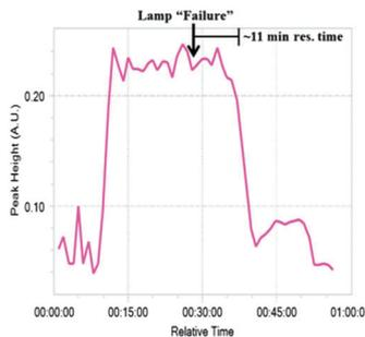
Fig. 4 The reaction exiting module 1 was monitored (FlowIR) at  $1033\text{ cm}^{-1}$ . To simulate an equipment error, the lamp was turned off during the reaction, resulting in cessation of the monitored peak following the  $\sim 11$  minute residence time of module 1.
