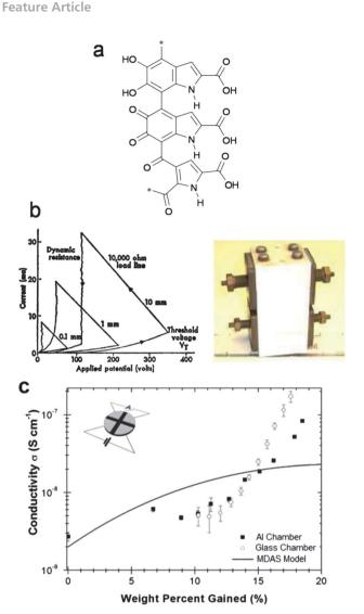
Fig. 3 (a) An example of the polymerized heterocycles that comprise melanin. (b) I–V characteristics and photograph of the original melanin "threshold switch" device fabricated by McGinness. (c) Relationship of conductivity to water uptake in melanin, from ref. 41
