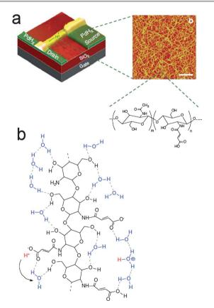
Fig. 4 (a) Bioprotonic transistor based on chitosan as a proton-conducting material. (b) Illustration of the Grotthus-like mechanism of proton conduction along the chitosan polysaccharide. Reproduced with permission from ref. 56.
