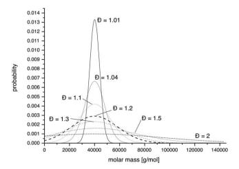
Fig. 2 Representation of theoretical Gaussian distributions of PHPMA with a degree of polymerisation of 300 ( $M_{\rm n}=40~{\rm kg~mol^{-1}}$ ) with a variation in the dispersity from 1.01, 1.04, 1.1, 1.2, 1.5 to 2.
