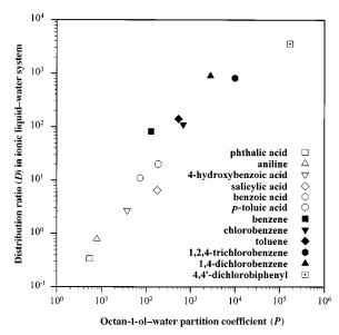
Fig. 1 Correlation of partitioning data between [BMIM][PF<sub>6</sub>]—water and octan-1-ol-water biphasic systems
