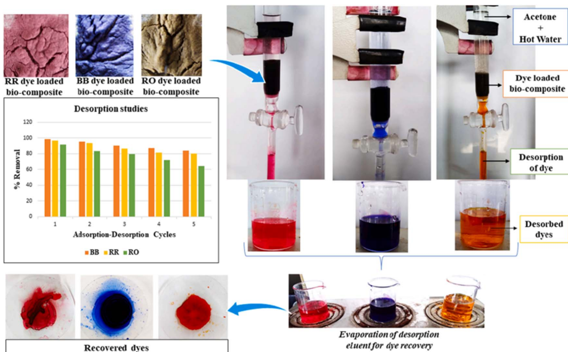
Fig. 7 Desorption studies of a dye-loaded bio-composite. 38
