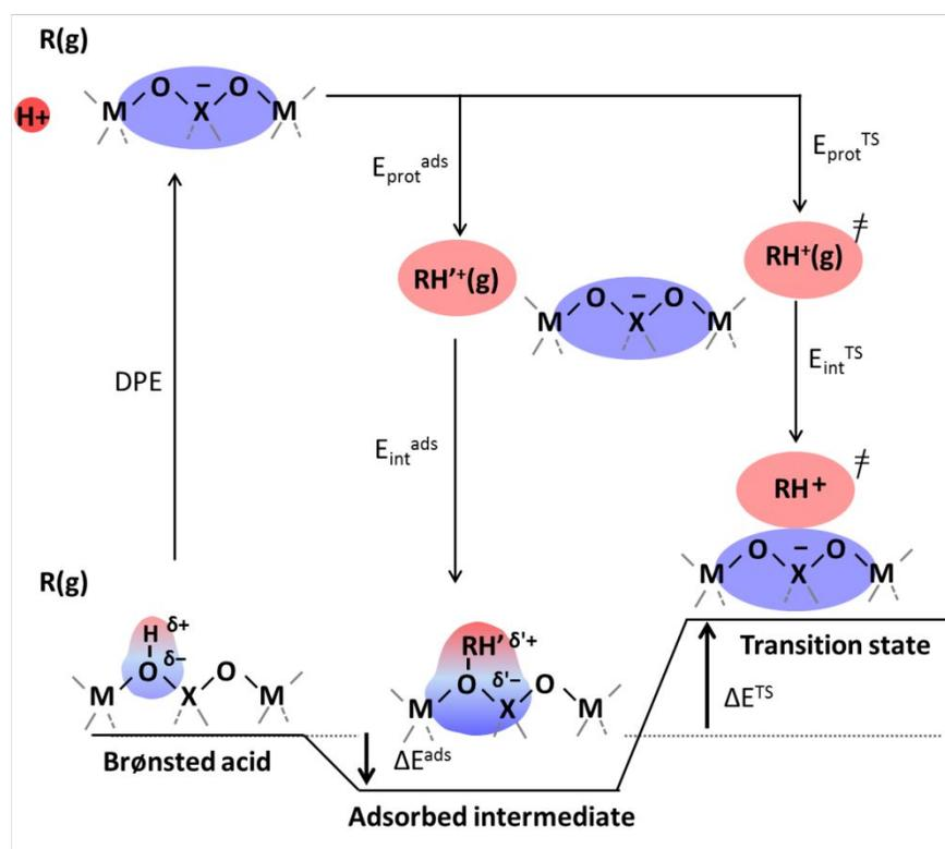
**Scheme 2.** A thermochemical cycle accounting for the thermodynamic properties of reactive intermediates ( $\Delta E^{ads}$ ) and transition states ( $\Delta E^{TS}$ ) involved in acid catalysis in terms of the DPE of the acid, the energies to form gaseous analogs of reactive intermediates and transition states from a free proton ( $E_{prot}^{ads}$ ,  $E_{prot}^{TS}$ ), and the energies of interaction of cations with the conjugate anion ( $E_{int}^{ads}$ ,  $E_{int}^{TS}$ ).
