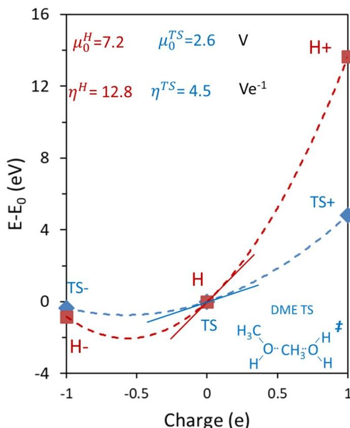
**Figure 10.** PW91 derived change in energy of H-atom and gaseous analog of DME formation transition state as a function of charge on the species. Dashed curves represent best fits to Equation 20. Solid lines represent local slopes. Derived from structures and methods in Ref. <sup>30</sup>.
