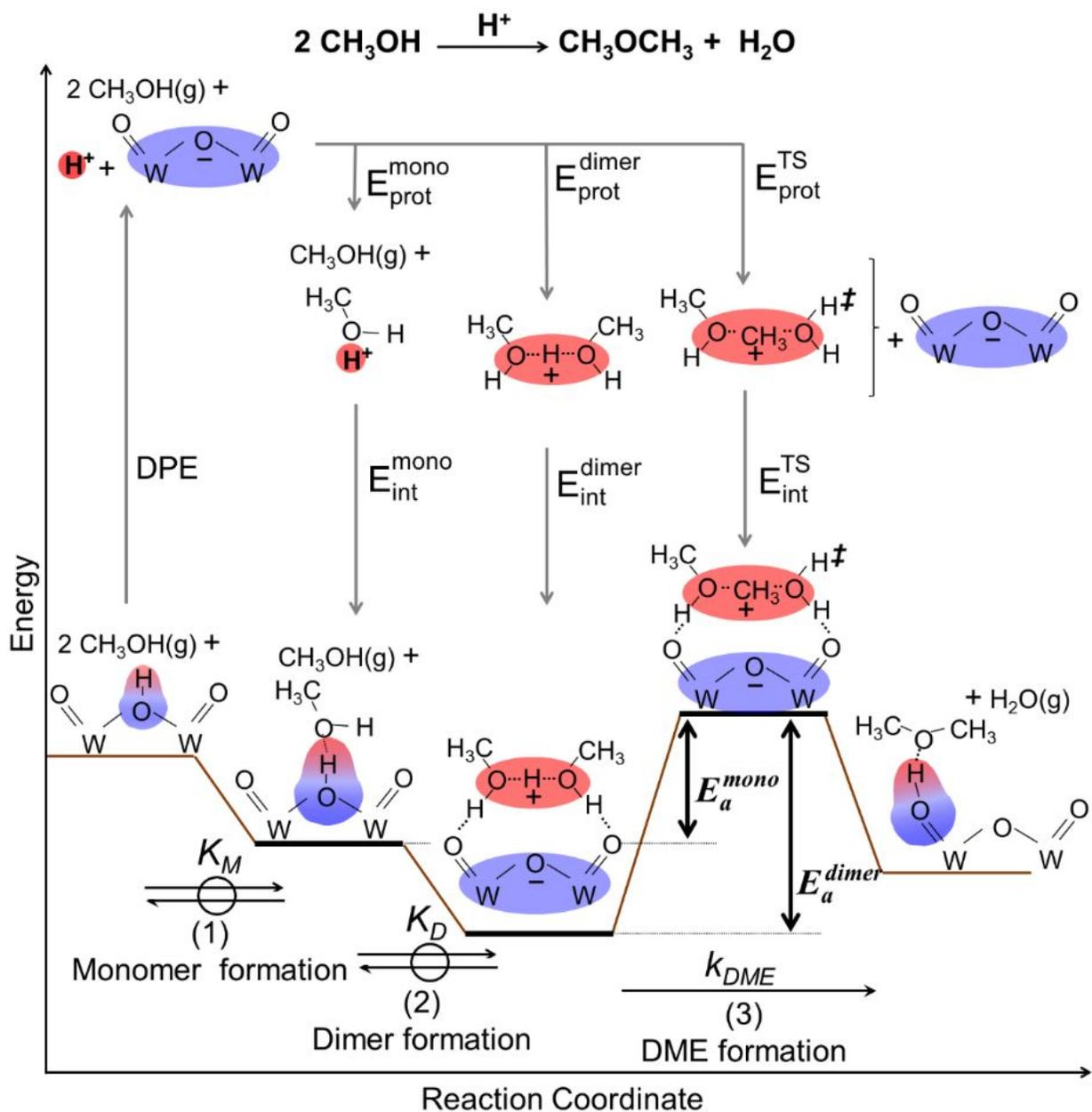
**Scheme 4.** Energy changes due to quasi-equilibrated steps forming adsorbed monomer and dimer intermediates from gaseous  $\text{CH}_3\text{OH}$  molecules and an irreversible step forming dimethyl ether via direct  $\text{CH}_3\text{OH}$  dehydration on Brønsted acids, and thermochemical cycles accounting for energies of surface species in terms of DPE,  $E_{\text{prot}}$  and  $E_{\text{int}}$ .
