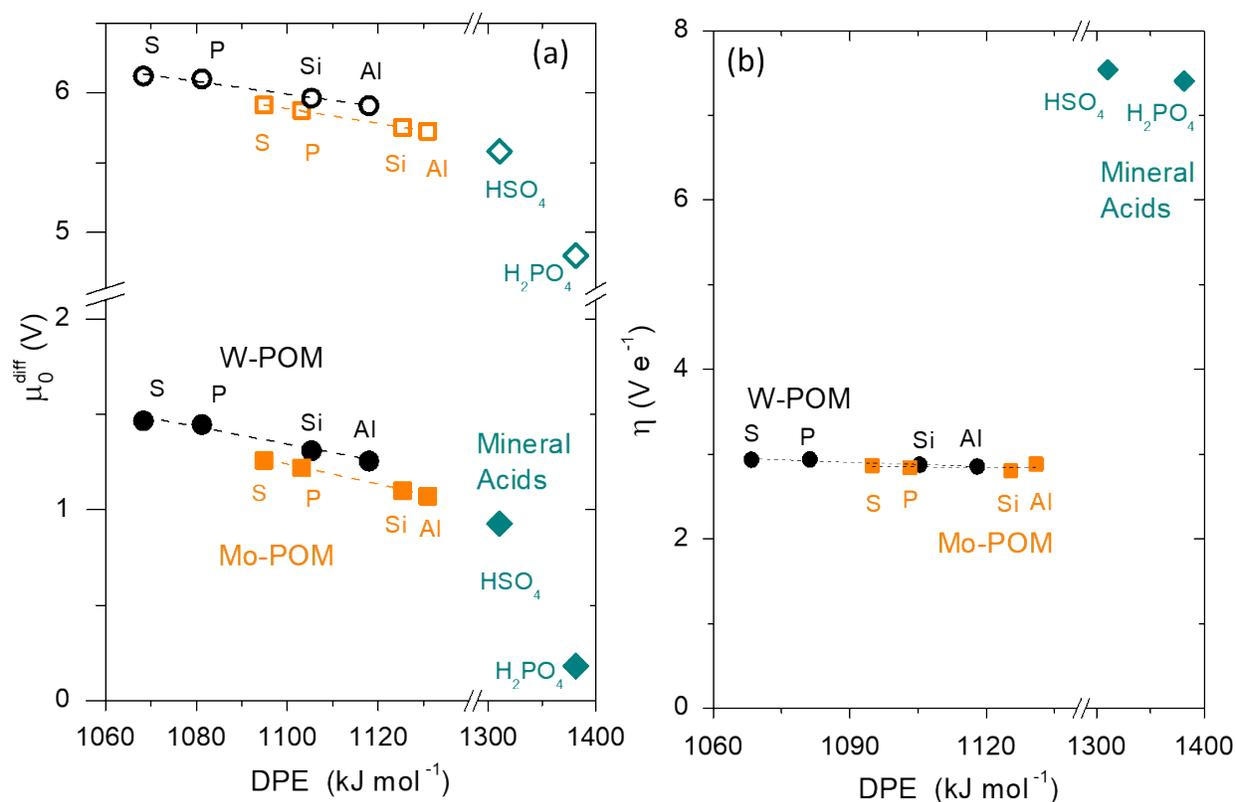
**Figure 11.** (a) Difference between chemical strengths of dehydrogenated POM clusters or mineral acids and H-atom ( $\mu_0 - \mu_0^H$ ; closed symbols) or DME formation transition state ( $\mu_0 - \mu_0^{TS}$ ; open symbols) and (b) chemical hardness ( $\eta$ ) for POM clusters and mineral acids as a function of DPE. The  $\mu_0$  and  $\eta$  values are derived from Equations 21 and 22 using methods and structures reported in Ref. <sup>30</sup>.
