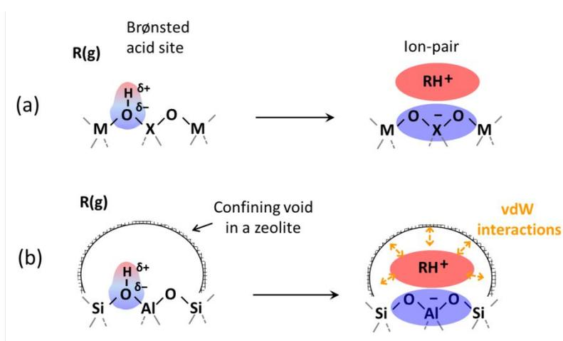
**Scheme 1.** Formation of cation-anion pairs in reactions of gaseous molecules ( $R(g)$ ) at solid Brønsted acid sites containing (a) unconfined heteroatom embedded in a metal oxide and (b) aluminosilicate zeolite with confining void environments. Identities of the heteroatom (X) and the metal atom (M) in (a) influence acid strength and ion-pair interactions while void structures influence van der Waals (vdW) stabilization of molecular species.
