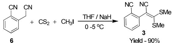
**Scheme 2:** Synthesis of 2-(1-cyano-2,2-bis(methylthio)vinyl)benzotrile
