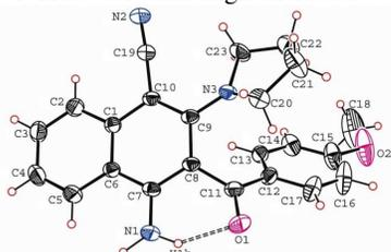
**Fig. 2.** ORTEP diagram of **10b** at 30% probability with atom numbering scheme. Only one molecule of the asymmetric unit comprising of two molecules is presented.
