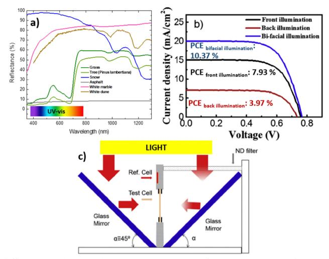
Fig. 3 (a) Reflectance data for different surface materials downloaded from Ecostress Spectral Library provided by the NASA Jet Propulsion Laboratory. 65 (b) J-V curves of a solid state BFDSC device by a back illumination, front illumination and bi-facial illumination (modified from ref. 68). (c) Schematic illustration of the light-splitting design in the bifacial cell tester, with simulated sunlight irradiating on both sides of the cell (modified image from ref. 68).
