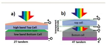
Fig. 14 Schematic example of (a) 2T tandem and (b) 4T tandem.
