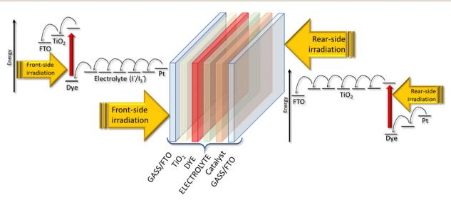
Fig. 2 Electron's motion in a BFDSC when irradiated from front and rear side (modified image from ref. 53).
