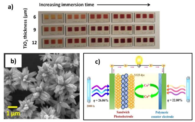
Fig. 8 (A) Comparison of fabricated WE with N719 dye considering the TiO<sub>2</sub> thickness and the immersion time. Reproduced and adapted from ref. 177. (B) SEM image of ZnO micro-flowers applied as SL from ref. 179 under Creative Commons BY-4.0 license (c) sandwich photoelectrode structure realized by ML-SL-ML from ref. 134 Copyright © 2022 American Chemical Society.
