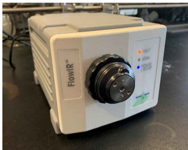
Fig. 1 Image of a FlowIR device that can be incorporated into a telescoped continuous flow sequence.
