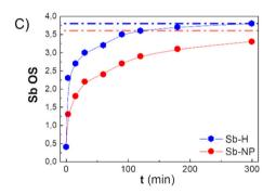
Fig. 5 In situ XANES spectra of (A) Sb-H and (B) Sb-NP in cell culture media (37 °C). (C) Time evolution of the oxidation state of Sb-H and Sb-NP obtained from the XANES analysis of the *in situ* measurements. The dotted lines represent the final oxidation state of the Sb-nanomaterials obtained by ex situ XANES. A continuous line does not represent a fitting of the data.
