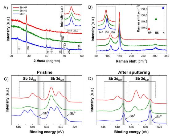
Fig. 3 (A) XRD diffractogram of the Sb-nanomaterials. Inset shows a detail of the 110 diffraction peaks. (B) Raman spectra of the nanomaterials. Insets show the details of the  $A_{1q}$  peak (left) and the Raman shift value of the  $A_{1q}$  peak (right). (C) XPS spectra of Sb nanomaterials as-synthesized and (D) after an Ar sputtering process in UHV.
