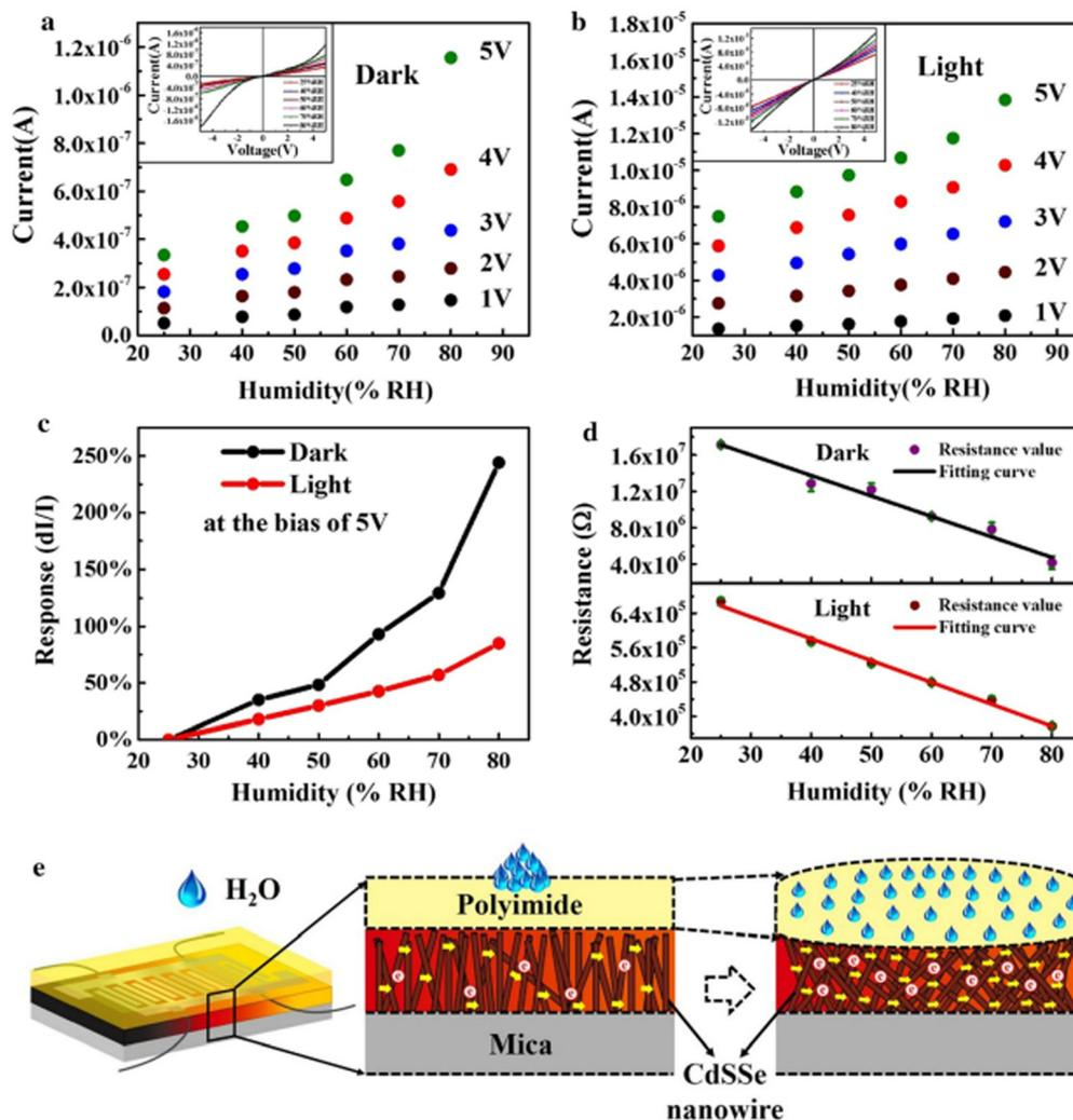
**Fig. 14** (a) Dark current and (b) photo-current at various humidity levels under different bias and the inset shows the IV characteristics in the dark (a) and light (b) at different relative humidity. (c) Relative humidity-dependent moisture responsivity of the sensor in dark and bright fields, respectively. (d) Resistance at various relative humidity of the sensor in dark and bright fields, respectively. (e) Schematic theoretical diagram of humidity sensing by the sensor.<sup>188</sup>
