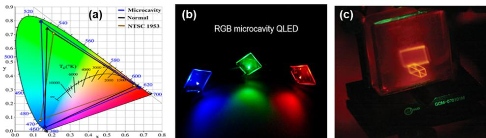
Fig. 18 (a) EL performances of best-performing RGB QLEDs. (a) CIE characteristics. (b) Image of RGB MQLEDs, Copyright © 2020, ACS Publications.<sup>372</sup> (c) Digital camera image for holographic reconstruction of cuboid under room light, Copyright © 2014, Wiley-VCH.<sup>373</sup>
