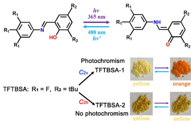
Fig. 10 Conversion of the enol form to the trans -keto form and vice versa upon UV light irradiation (up) and photochromic and non-photochromic behaviour of the polymorphic forms TFTBSA-1 and TFTBSA-2, respectively. tBu = tert -butyl. Reprinted (used in part) with permission from ref. 75. Copyright 2021 American Chemical Society.
