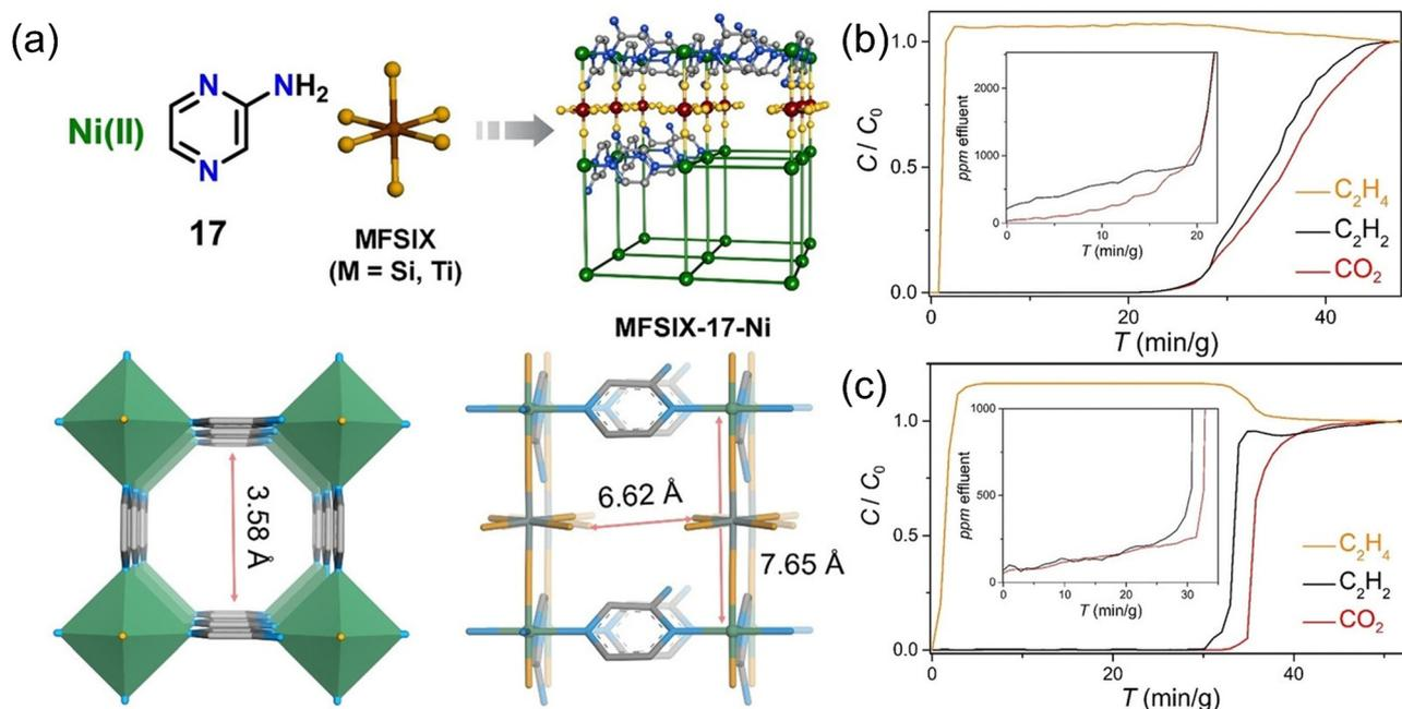
Fig. 8 (a) Structure and channel diagram of TIFSIX-17-Ni. Ambient temperature (298 K) and pressure (1 bar) experimental dynamic column breakthrough curves for  $\text{C}_2\text{H}_4/\text{C}_2\text{H}_2/\text{CO}_2$  (1 : 1 : 1, v/v/v) ratio by a sorbent bed filled with (b) SIFSIX-17-Ni and (c) TIFSIX-17-Ni. Reproduced with permission from ref. 67. Copyright © 2021, Wiley-VCH GmbH.
