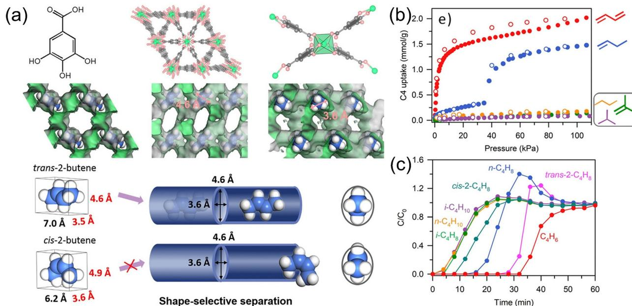
**Fig. 11** (a) Structure, channel, and separation of *trans*- and *cis*-2-butene of M-gallate. (b) Adsorption isotherms of *trans*-2-butene, *cis*-2-butene, 1,3-butadiene, 1-butene, iso-butene, *n*-butane, and iso-butane on Co-gallate at 298 K. (c) Mixture breakthrough curves on Mg-gallate for 1,3-butadiene/1-butene/iso-butene/*n*-butane/iso-butane/*trans/cis*-2-butene/He (20/10/10/5/1/2/2/50) at 298 K. Reproduced with permission from ref. 91. Copyright © 2020, American Chemical Society.
