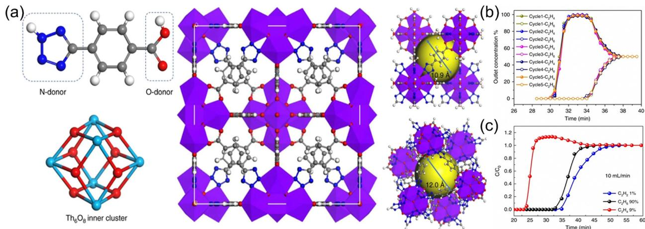
Fig. 5 (a) A Th-MOF (Azole-Th-1) based on  $\text{Th}_6$  secondary building units and tetrazolyl groups. (b)  $\text{C}_2\text{H}_6/\text{C}_2\text{H}_4$  (50/50, v/v) binary mixture separation for five cycles. (c)  $\text{C}_2\text{H}_6/\text{C}_2\text{H}_4/\text{C}_2\text{H}_2$  (90/9/1, v/v/v) ternary mixture separation. Reproduced with permission from ref. 54. Copyright © 2020, Springer Nature Publishing AG.
