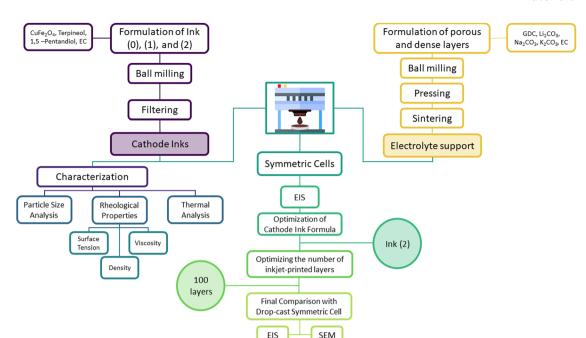
Experimental steps of fabrication, characterization, and optimization for an inkjet-printed CuFe<sub>2</sub>O<sub>4</sub> symmetric cell.
