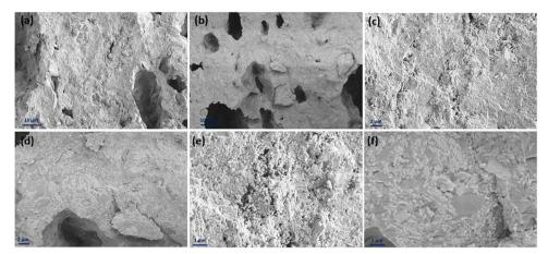
Fig. 12 Cross-sectional SEM images of (a), (c) and (e) 100-layers and (b), (d) and (f) drop-cast porous NLK-GDC symmetric cells in  $1.23k \times$  (a and b),  $3.71k \times$  (c and d), and  $9.77k \times$  (e and f) magnifications.
