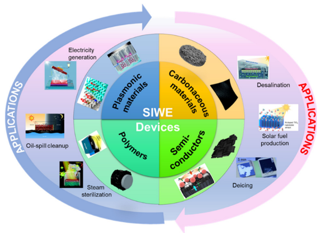
Fig. 6 Schematic diagram illustrating various potential applications of the SIWE device. Plasmonic materials. Reproduced by permission. 8,30 Copyright 2016, Springer Nature. Copyright 2016, American Chemical Society|| Carbonaceous materials. Reproduced by permission. 4,108 Copyright 2014, Nature. Copyright 2017, Royal Society of Chemistry|| Semiconductor. Reproduced by permission. 48,109 Copyright 2019, Royal Society of Chemistry. Copyright 2020, American Chemical Society|| Polymers. Reproduced by permission. 10,60 Copyright 2018, Nature. Copyright 2015, Wiley-VCH|| Desalination. Reproduced by permission. 110 Copyright 2021, Royal Society of Chemistry|| Solar fuel production. Reproduced by permission. 111 Copyright 2009, American Chemical Society|| De-icing. Reproduced by permission. 112 Copyright 2018, American Association for the Advancement of Science|| Steam generation. Reproduced by permission. 113 Copyright 2017, Royal Society of Chemistry|| Oil-spill cleanup. Reproduced by permission. 114 Copyright 2020, Royal Society of Chemistry|| Electricity generation. Reproduced by permission. 115 Copyright 2018, Elsevier.
