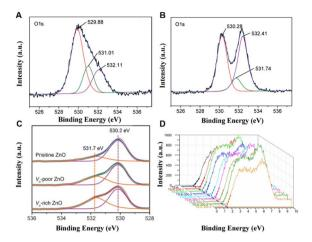
Fig. 10 (A) XPS of pure TiO<sub>2</sub> nanorods and (B) TiO<sub>2</sub> nanorods with Cu doping. 110 Copyright © 2010 American Chemical Society. (c) XPS of V<sub>O</sub>-rich ZnO.<sup>112</sup> Copyright © 2012 American Chemical Society. (D) XPS valence band spectra of black TiO<sub>2</sub> samples.<sup>113</sup> Copyright © 2018 Elsevier Inc.
