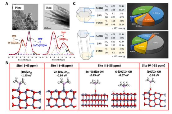
Fig. 6 (A) 31P NMR spectra of TMP-adsorbed plate-/rod-like ZnO crystallites. (B) DFT simulation of the adsorption configuration and energy of TMP on Zn<sub>3C</sub> (I and II) and proton (III and IV) species. (C) Distribution, concentration, and percentage of various surface features on plate-/rod-like ZnO revealed by TMP-31P NMR.88 Copyright © 2016 American Chemical Society.
