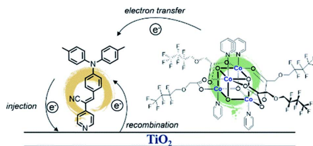
Fig. 24 Representation of the photosynthetic assembly proposed by Meyer and co-workers based on a triphenylamine photosensitizer and a tetracobalt cubane WOC. Reprinted from ref. 129 with permission from the Royal Society of Chemistry, copyright 2022.
