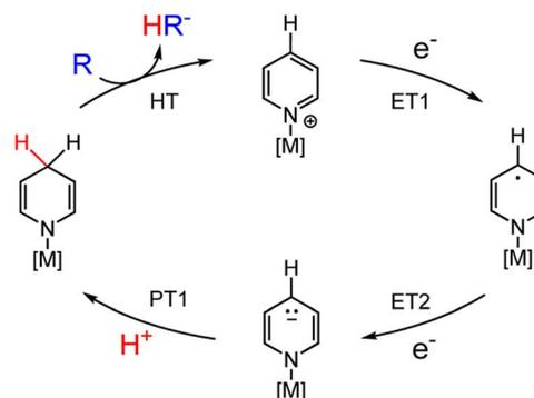
**Scheme 2** Possible catalytic cycle to enable electrochemical regeneration of  $DHP^-$  for hydride transfer (HT) reactions. ET = electron transfer; PT = proton transfer. In some cases, the ordering of the ET2 and PT1 elementary steps is reversed.
