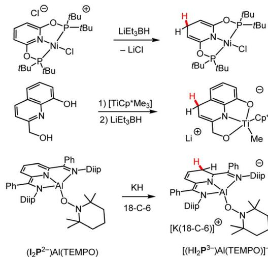
**Scheme 5** Examples of syntheses of M-DHP<sup>-</sup> complexes by the addition of various metal hydrides.<sup>84,85,89</sup> Cp\* = pentamethylcyclopentadienyl; Diip = 2,6-diisopropylphenyl; 18-C-6 = 18-crown-6 ether; I<sub>2</sub>P = diiminepyridyl; TEMPO = (2,2,6,6-tetramethylpiperidin-1-yl)oxyl.
