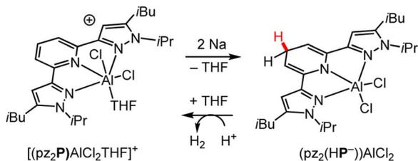
**Scheme 6** Synthesis of  $\text{pz}_2(\text{HP}^-)\text{AlCl}_2$ ,<sup>91</sup> where pz is the substituted pyrazolyl shown and P is the pyridyl ligand backbone.  $\text{HP}^-$  denotes the dihydropyridinate form, which is analogous to  $\text{DHP}^-$ . Protons are believed to be scavenged from ligand equivalents during reduction by Na.
