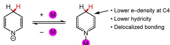
Scheme 9 Common changes to DHP<sup>-</sup> upon coordination of a metal atom, M, at the pyridyl N atom.
