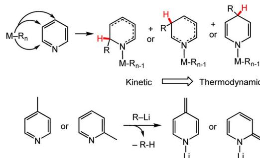
**Scheme 3** (Top) The general reaction pathway for alkylation to make either 1,2-DHP<sup>-</sup>, 1,3-DHP<sup>-</sup> or 1,4-DHP<sup>-</sup> metal complexes, including the relative stability of the alkylation products. M = metal centre; R<sub>n</sub> = alkyl group. (Bottom) Deprotonation of acidic functional groups is a possible side reaction with metal-alkyl reagents;<sup>60</sup> avoiding this side reaction is a common challenge in the synthesis of M-DHP<sup>-</sup> compounds.
