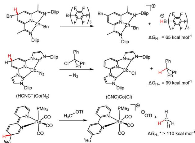
**Scheme 12** HTs from M-DHP<sup>-</sup> complexes.  $\Delta G_{H^-}$  are the reported for the hydride acceptors.<sup>18,86,109,110</sup> Bn = benzyl; Diip = 2,6-diisopropylphenyl; CNC = tridentate pincer ligand coordinating at 2 C and 1 N, as shown; OTf = triflate.
