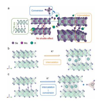
Fig. 1 (a) Schematic illustration of the modulation of Se–Se bonds. (b and c) Crystal structure and mechanism of MoSe<sub>2</sub> and MoSe<sub>2+x</sub>, respectively. Purple atoms represent selenium, pink atoms represent molybdenum, and green atoms represent potassium.
