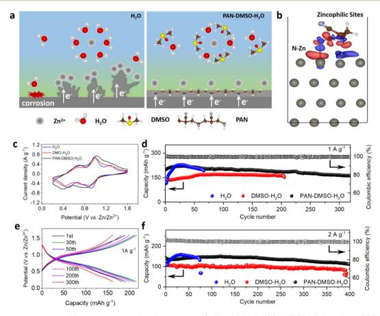
Fig. 5 (a) Schematic illustration of Zn deposition with the pristine aqueous (left) and PAN-DMSO- $H_2O$  (right) electrolytes. (b) Side view of the charge density difference at the Zn-PAN interface. (c) CV profiles at a scan rate of 0.1 mV s<sup>-1</sup> in different electrolytes. (d) Cycling performance at a current density of 1 A g<sup>-1</sup> and (e) the corresponding galvanostatic charge-discharge curves. (f) Cycling performance at a current density of 2 A g<sup>-1</sup>.
