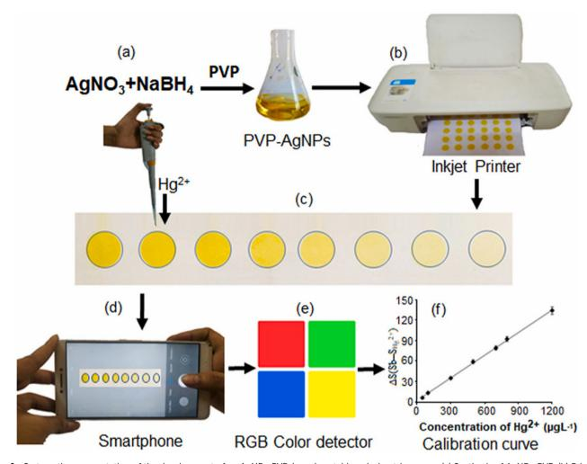
Fig. 6 Systematic representation of the development of an AgNPs-PVP-based portable colorimetric sensor. (a) Synthesis of AgNPs-PVP. (b) Printing of AgNPs in filter paper. (c) Pipetting Hg<sup>2+</sup> in an AgNP sensing probe. (d) Image captured using a smartphone. (e) RGB value analyzed using ImageJ software. (f) The result as a calibration curve [this figure has been reproduced from ref. 60 with permission from Elsevier Sciences, copyright 2021].
