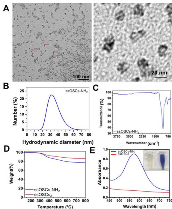
**Fig. 1** Characterization of the breakable ssOSCs-NH<sub>2</sub>. (A) Transmission electron microscopy images of the ssOSCs functionalized with NH<sub>2</sub> groups. (B) DLS analysis, (C) FTIR spectrum, (D) TGA of ssOSCs-NH<sub>2</sub> compared to ssOSCs. (E) Kaiser test for determining primary amines with the maximum absorption peak at 570 nm.
