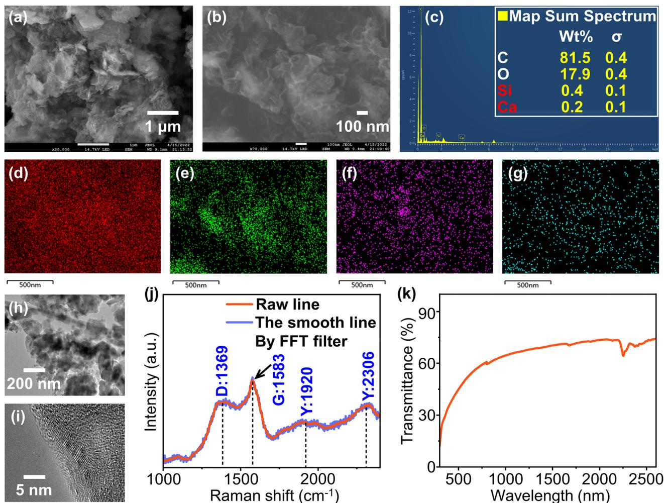
**Fig. 2** (a) SEM image at a scale of 1  $\mu\text{m}$ . (b) SEM image at a scale of 100 nm. (c) Atomic ratio of  $\gamma$ -GY NSs. EDS images of  $\gamma$ -GY NSs corresponding to (d) C, (e) O, (f) Si and (g) Ca, respectively. (h) TEM image and (i) HRTEM image of  $\gamma$ -GY NSs. (j) Raman spectrum of  $\gamma$ -GY NSs. (k) VIS-IR transmission spectrum of  $\gamma$ -GY NSs.
