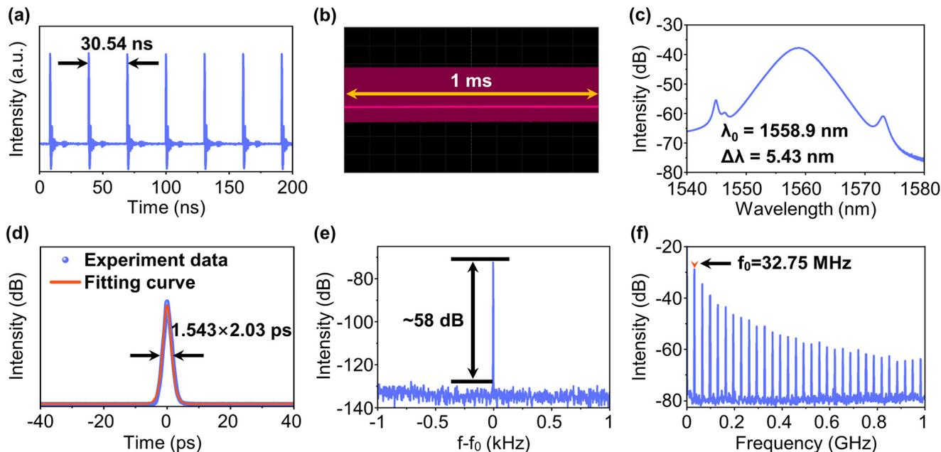
**Fig. 8** (a) Temporal pulse trains and (b) oscilloscope trace within 1 ms. (c) The optical spectrum. (d) Autocorrelation trace with  $\text{sech}^2$  pulse profile. (e) RF spectrum over a 2 kHz span with a resolution bandwidth of 1 Hz at the fundamental frequency and (f) the wideband RF spectrum with 100 kHz resolution.  $\Delta\lambda$ : 3 dB bandwidth;  $f_0$ : fundamental frequency.
