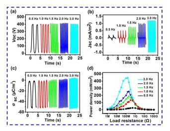
**Fig. 3** Electrical output performance of the 2# MCH-TENG at different contact frequencies. (a–c) Electrical output ( $V_{\rm oc}$ ,  $J_{\rm sc}$  and  $\sigma_{\rm sc}$ ). (d) Power densities under different external loads.
