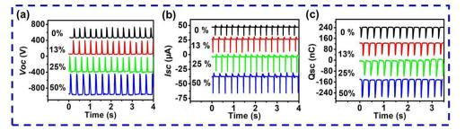
Fig. 4 (a)  $V_{\rm oc}$ , (b)  $I_{\rm sc}$  and (c)  $Q_{\rm sc}$  of the 2# MCH-TENG under stretching strain from 0% to 50%.
