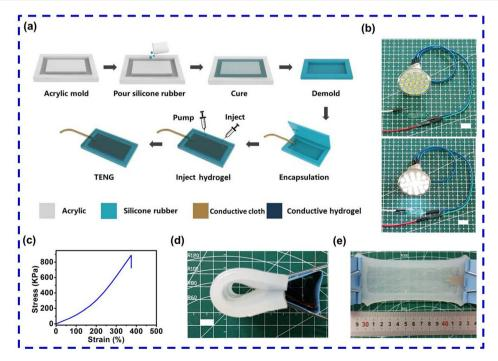
Fig. 1 (a) Schematic diagram of the detailed fabrication process of the MCH-TENG. (b) Photographs of the circuit comprising of the MCH and LED light (V = 8 V; top: open circuit; bottom: closed circuit). (c) The stress-strain curve of the silicone rubber cube ( $59 \times 10 \times 2 \text{ mm}^3$ ). (d and e) Photographs of the MCH-TENG at bending (d) and stretching states (50%). (All scale bar = 1.0 cm.)
