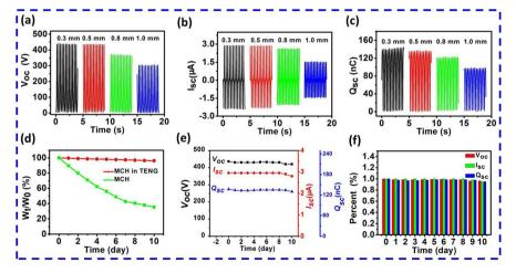
Fig. 5 The outputs of  $V_{\rm oc}$  (a),  $I_{\rm sc}$  (b) and  $Q_{\rm sc}$  (c) of the MCH-TENGs with different thicknesses of silicone rubber. (d) Weight changes of the MCH in the MCH-TENG and open air as a function of storage time for 10 days. (e) Outputs and (f) retention rate of  $V_{\rm oc}$ ,  $I_{\rm sc}$  and  $Q_{\rm sc}$  of the MCH-TENG as a function of storage time for 10 days.
