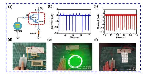
Fig. 8 (a) Schematic diagram of the MCH-TENG and a Darlington transistor connected circuit. (b and c)  $I_{sc}$  of the 2# MCH-TENG without (b) and with (c) the Darlington transistor under hand tapping. (d and e) The circuit connected to different loads: (d) electronic counter ( $V_{cc} = 5$  V); (e) LED light strip ( $V_{cc} = 12$  V); (f) LED light board ( $V_{cc} = 18$  V).
