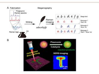
Fig. 2 The patterning process of writing. (A) Pen writing. Reproduced with permission from ref. 36. Copyright 2021 John Wiley & Sons, Inc. (B) Laser writing. Reproduced with permission from ref. 37. Copyright 2021 American Chemical Society.
