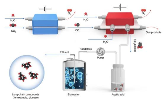
Fig. 1 Schematic illustration of an artificial synthesis system for glucose. CO2 was first converted to acetic acid through a two-step electrochemical reaction. The generated acetic acid was then fermented in a bioreactor as a microbial substrate to produce long-chain compounds such as glucose (ref. 2).
