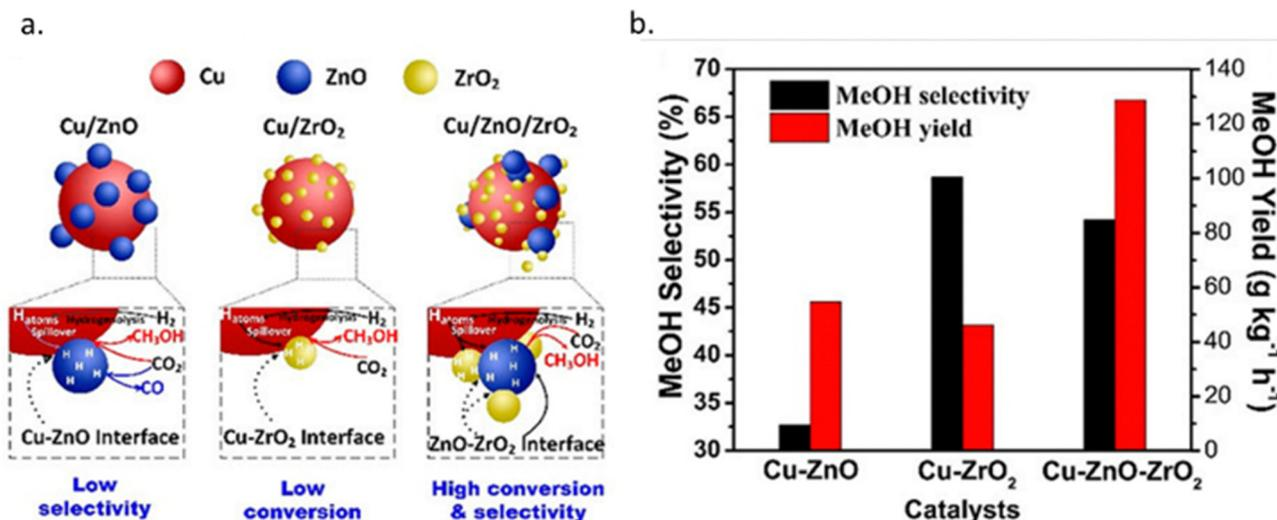
Fig. 5 (a) Schematic diagram of the CO<sub>2</sub> hydrogenation process over Cu–ZnO, Cu–ZrO<sub>2</sub> and Cu–ZnO–ZrO<sub>2</sub> catalysts. (b) Methanol yields and methanol selectivity of Cu–ZnO, Cu–ZrO<sub>2</sub> and Cu–ZnO–ZrO<sub>2</sub> catalysts. Reprinted with permission from ref. 78. Copyright 2019 American Chemical Society (<https://pubs.acs.org/doi/full/10.1021/acscatal.9b01943>).
