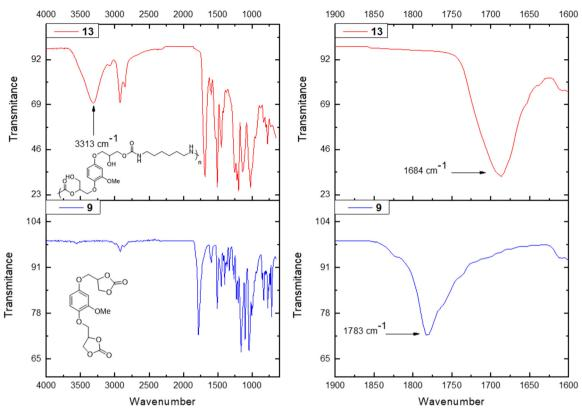
Fig. 1 FT-IR spectrum of hydroquinone-based PHUs (13) prepared from hydroquinone-based bis-carbonate (9) (left), zoom of carbonyl stretching region of hydroquinone-based PHUs (13) prepared from hydroquinone-based bis-carbonate (9) (right).
