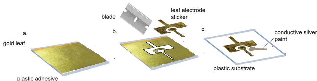
**Fig. 5** Pure gold leaf electrode fabrication does not require specialized equipment. (a) Gold leaf adhesive is applied to a side of Fellowes. (b) Gold leaf is applied to the adhesive and cut. (c) The gold leaf stickers are peeled off and placed on a transparency film. Conductive silver paint is applied to the leads of all three electrodes. Figure reproduced and adapted from ref. 95 (Zamani *et al.*, 2020) with permission. Copyright American Chemical Society 2021.
