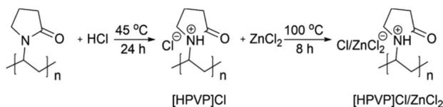
Fig. 19 Scheme of synthesis of Brønsted–Lewis [HPVP]Cl/ZnCl<sub>2</sub> deep eutectic solvent polymer via quaternization of PVP. Reproduced from ref. 65 with permission from Elsevier, 2023.
