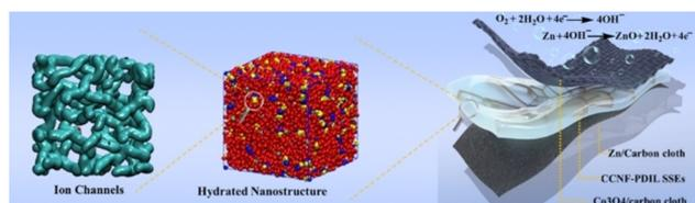
**Fig. 15** Safe, environmentally benign, hierarchically nanostructured CCNF-PDIL solid-state electrolytes with reinforced concrete architecture are constructed by nanoconfined polymerization of dual-cation ionic liquid (PDIL, concrete) within a robust three-dimensional porous cationic cellulose nanofiber matrix (CCNF, reinforcing steel) for flexible zinc–air batteries. Reproduced from ref. 49 with permission from Wiley, 2022.
