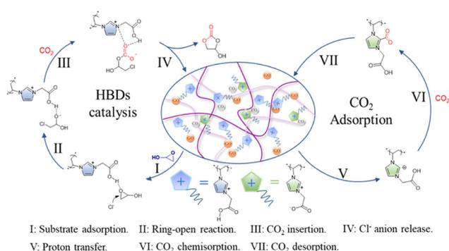
**Fig. 8** Mechanism diagram of the cycloaddition reaction between glycidyl and CO<sub>2</sub> catalyzed by P-DVB-CE/CCLMCl. Reproduced from ref. 21 with permission from Elsevier, 2023.
