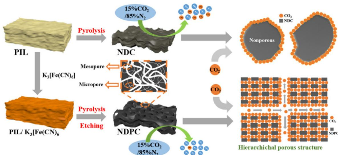
Fig. 10 Preparation of N-doped hierarchically porous carbon derived from PIL and potassium ferricyanide and mechanism diagram of CO<sub>2</sub> adsorption on NDC and NDPC adsorbents. Reproduced from ref. 26 with permission from ACS, 2021.
