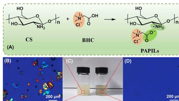
**Fig. 2** The synthesis of novel material: the protonation of the amino groups in CS by the carboxyl groups in BHC to form PAPILs in water (A). Optical and polarizing images of 3 wt% CS in water (B, left in C) and in 0.3 M BHC aqueous solution (right in C and D) – the PAPILs solution is viscous and transparent. Reproduced from ref. 9 with permission from Elsevier, 2023.
