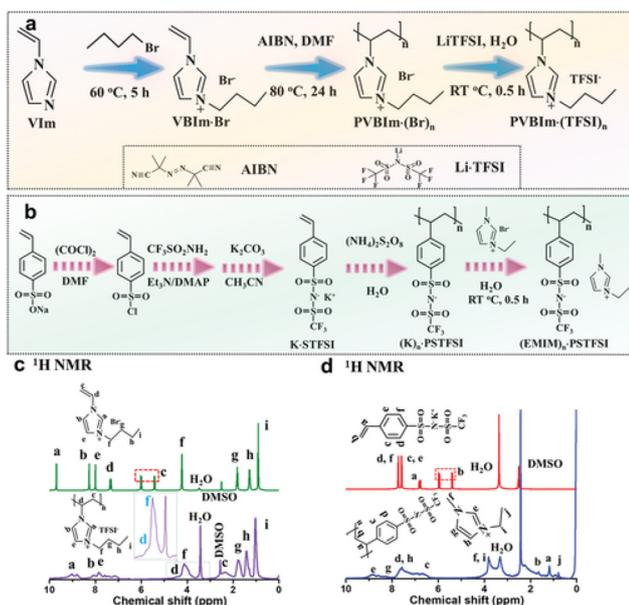
**Fig. 16** Synthesis and characterization of two poly(ionic liquids). (a) Synthetic scheme of PVBlm-(TFSI)<sub>n</sub>. (b) Synthetic scheme of (EMIM)<sub>n</sub>-PSTFSI. (c) <sup>1</sup>H NMR for VBlm-Br and PVBlm-(TFSI)<sub>n</sub>. (d) <sup>1</sup>H NMR for K-STFSI and (EMIM)<sub>n</sub>-PSTFSI. Reproduced from ref. 54 with permission from Wiley, 2021.
