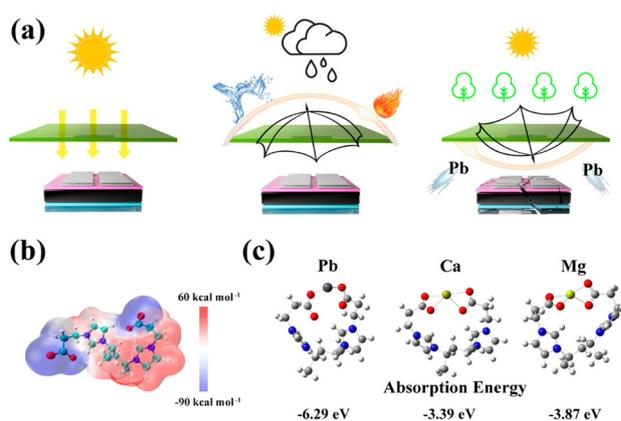
**Fig. 12** (a) Ambidextrous protective shield manufactured by PPVI-TFSI. (b) Electrostatic potential distribution for PPVI-TFSI. (c) Optimized structures and absorption energy for PIL toward different cations. Reproduced from ref. 41 with permission from ACS, 2023.
