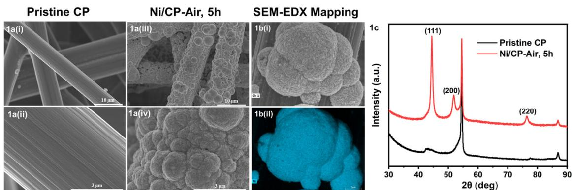
**Fig. 1** (a) (i & ii) SEM images of pristine carbon paper (CP); (iii & iv) CP after electroplating from a 40 mM solution of  $\text{NiCl}_2 \cdot 6\text{H}_2\text{O}$  for 5 h under air (Ni/CP-Air); (b) (i & ii) SEM & EDX elemental mapping of Ni/CP-Air; (c) XRD spectrum of pristine CP & Ni/CP-Air.
