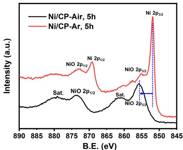
**Fig. 2** XPS comparison between Ni/CP-Air (black line) & Ni/CP-Ar (red line). The Ni/CP-Air electrode was prepared under air atmosphere & the CP was undergone 5 h electroplating in 40 mM of NiCl<sub>2</sub>·6H<sub>2</sub>O in methanol at 10 mA. The Ni/CP-Ar electrode was prepared under Ar atmosphere & the CP was undergone 5 h electroplating in 40 mM of NiCl<sub>2</sub>·6H<sub>2</sub>O in methanol at 10 mA.
