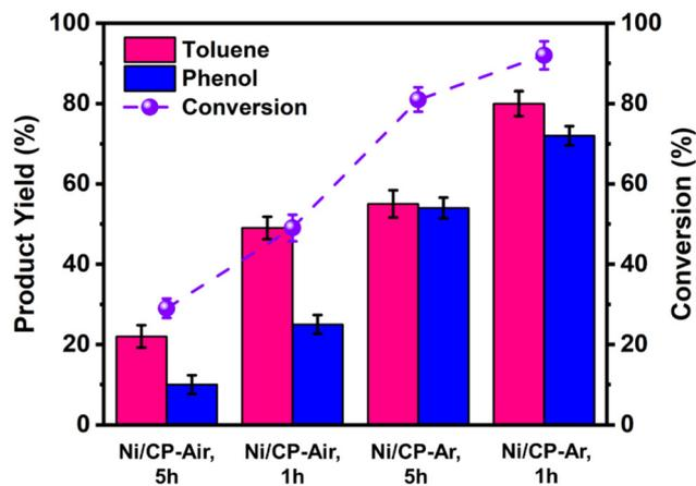
**Fig. 3** Product yields (left Y-axis) and conversion (right Y-axis) results of ECH experiments of benzyl-phenyl ether (BPE) carried out with different cathode materials listed on the X-axis. All cathode materials were prepared by electroplating NiCl<sub>2</sub>·6H<sub>2</sub>O onto carbon paper (CP), under air or argon, and for 1 h or 5 h. ECH of entries 1 & 2 were performed under air, 3 & 4 were performed under argon.
