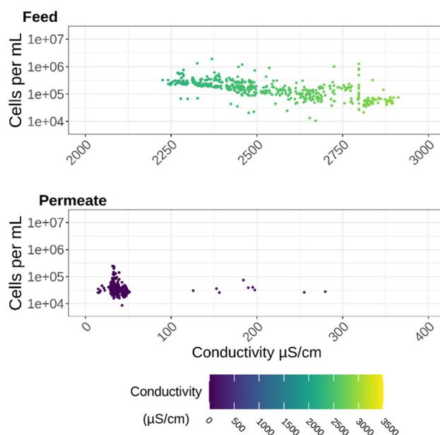
**Fig. 5** The measured conductivity values of the feed (top) and permeate (bottom) stream plotted in function of the cell densities. There is no clear visual correlation between conductivity values and cell density.
