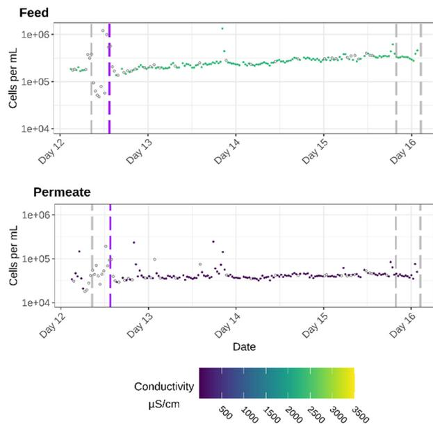
**Fig. 4** Overview of the cell densities (cells per mL) and conductivity values (colour-scale) in the feed (top) and permeate (bottom) stream right before and during the days after the ultrasound treatment (purple dashed line). The grey lines mark flushes. If the pilot is not in operation conductivity was not measured and therefore given in grey (hollow points).
