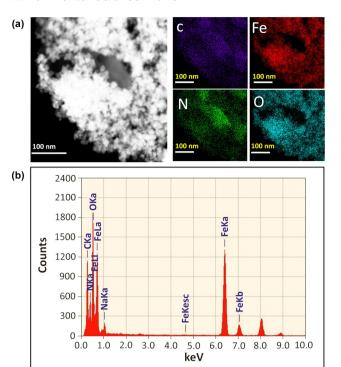
Fig. 4 (a) SEM and EDS elemental mapping of C, Fe, N, and O of M-g-CN. (b) EDX spectra of M-g-CN nanocomposite with element arrangements.
