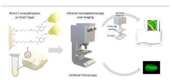
the ATA-117 transaminase 1 Schematic overview of immobilization on EziG carriers and the microscopic characterization of the resulting biocatalysts.
