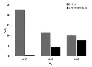
Fig. 7 GC-MS results of the transamination of 1-phenoxypropan-2one in the presence of isopropyl amine as an amine donor, catalyzed by His<sub>6</sub>-ATA-117 immobilized on EziG<sup>1</sup>-Opal at different a<sub>w</sub> values. Reaction conditions: 1 mL toluene, 250 mM isopropyl amine, 100 mM 1-phenoxypropan-2-one, 35 °C, 150 rpm, overnight. The  $a_{\rm w}$  values were obtained and measured as described in the Experimental section.
