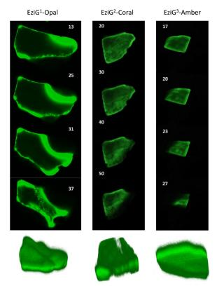
Fig. 5 2D images (40×) of different layers of EziG<sup>1</sup>, EziG<sup>2</sup> and EziG<sup>3</sup> carriers obtained by acquiring 3D image stacks with scanning confocal microscopy showing the FITC labelled His6-ATA-117 distribution (samples were pretreated with NaP buffer before drying pretreatment 1) Row below: 3D reconstruction of the shown carriers
