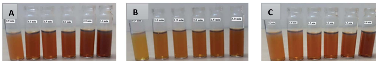
Fig. 3 Color change observed during microwave irradiation of the reaction mixture containing (a) AgNPs-HCL, (b) AgNPs-HCF, and (c) AgNPs-HCS, where the abbreviations HCL, HCF, and HCS stand for leaf, fruit and stem extracts, respectively, from the plant Hyptis capitata (HC).
