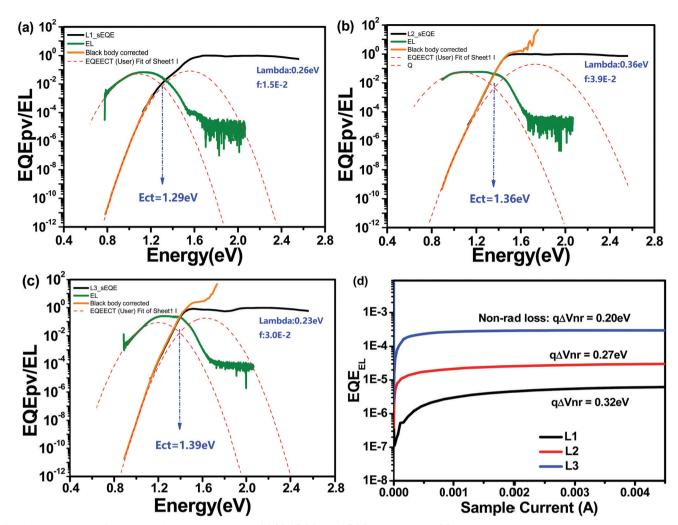
Normalized sEQE spectra of solar cells based on L1 (a), L2 (b), and L3 (c), and EL curves (d).
