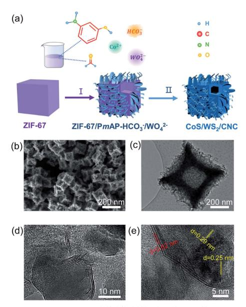
Fig. 1 (a) Schematic illustration of the fabrication pathway of CoS/WS<sub>2</sub>/CNC. (b) SEM, (c and d) TEM, and (e) high-resolution TEM images of CoS/ WS<sub>2</sub>/CNC-1.
