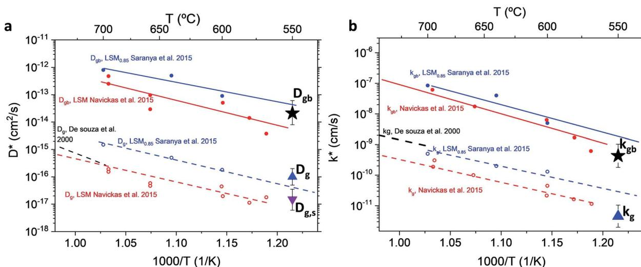
Fig. 3 Diffusivity (a) and surface exchange coefficient (b) for nanocrystalline LSM measured by APT and compared to literature values (for stoichiometric and B-site deficient (LSM<sub>0.85</sub>) materials).<sup>13,14,29</sup> Values from Saranya *et al.* 2015 (ref. 14) have been updated using the FEM model introduced by the authors in Saranya *et al.* 2018 (ref. 18). The error bars are calculated from the sensitivity analysis described in ESI Note 2.†
