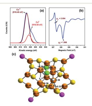
Fig. 5 (a) Deconvoluted Cu LMM Auger spectrum of the  $Cu_{18}$  NC, (b) EPR spectrum of the  $Cu_{18}$  NC, and (c) Bader charge analysis of the optimized  $Cu_{18}$  NC. Color legend: Cu, orange; S, yellow; P, magenta; Cl, green; H, white. For clarity, all phenyl and adamantane groups are omitted.
