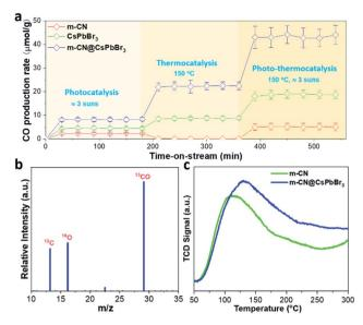
Fig. 3 (a) The CO<sub>2</sub> reduction to CO performance under the three conditions of photocatalysis, thermocatalysis and photo-thermocatalysis. For the latter two, the temperature is set to 150 °C; (b) mass spectrometry (MS) result of  $^{13}\text{CO}$  produced over m-CN@CsPbBr<sub>3</sub> from the  $^{13}\text{CO}_2$  isotope experiment under thermocatalysis (*m/z*, mass/charge ratio); (c) CO<sub>2</sub>-TPD results of the reference m-CN and the m-CN@CsPbBr<sub>3</sub> catalyst.
