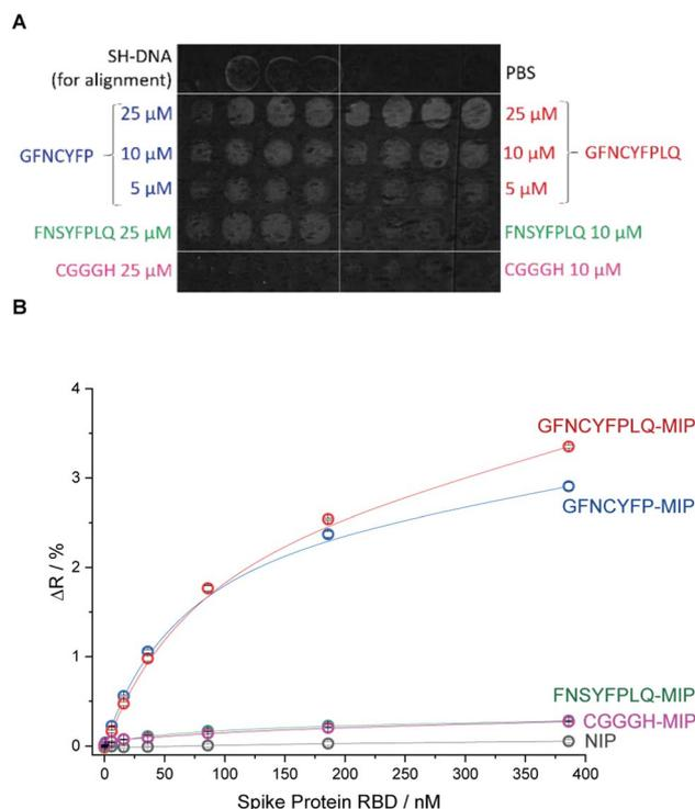
Fig. 2 (A) The SPR image and microspotting layout of the epitope-imprinted polymer microarray. Each peptide concentration was spotted in triplicates. The diameter of the spots is ca. 500  $\mu\text{m}$  with 420  $\mu\text{m}$  spacing. (B) RBD binding to the different peptide-imprinted polyscopoletin spots.
