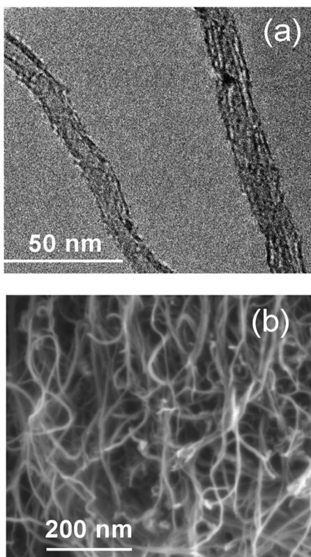
**Fig. 14** TEM (a) and SEM (b) microphotographs of MWCNT found in the products of CO<sub>2</sub> electrolysis conducted in borate (Li<sub>1.5</sub>Na<sub>1.5</sub>BO<sub>3</sub>) and eutectic carbonate (Li<sub>1.24</sub>K<sub>0.76</sub>CO<sub>3</sub>) blend (1 : 1 mol/mol) at 550 °C.
