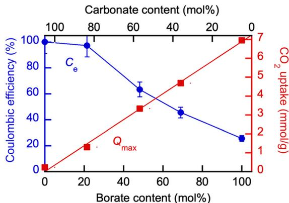
**Fig. 12** Effect of the molten borate/carbonate blend composition on the Coulombic efficiency ( $C_e$ ) of the  $CO_2$  electrolysis and maximum  $CO_2$  uptake ( $Q_{max}$ ) at 550 °C. Borate:  $Li_{1.5}Na_{1.5}B_2O_3$ ; eutectic Li, K carbonate:  $Li_{1.24}K_{0.76}CO_3$ . For  $Q_{max}$  determination detail, see legend to Fig. 6.
