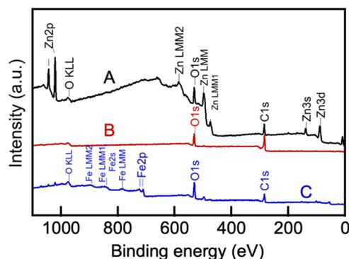
**Fig. 10** XPS spectra of the original galvanized steel electrode (A), the same electrode utilized in the  $\text{CO}_2$  electrolysis at 550 °C in molten Li, K borate/Li, Na carbonate (1 : 1 mol/mol) blend (B), and the same electrode after cleaning its surface of the CNT deposited during the electrolysis (C). For electrolysis conditions, see Experimental.
