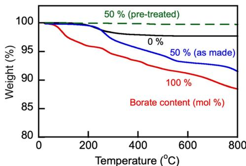
**Fig. 2** TGA heating ramp (10 °C min<sup>-1</sup>) of as-made carbonate ( $\text{Li}_{1.24}\text{K}_{0.76}\text{CO}_3$ ), borate ( $\text{Li}_{1.5}\text{Na}_{1.5}\text{BO}_3$ ) and as-made and pre-treated blend (1:1 mol/mol, sample no. 3 in Table 1) in nitrogen atmosphere. The blend sample was pre-treated by its equilibration at 600 °C in N<sub>2</sub> atmosphere for 1 h. Numbers stand for nominal initial content of borate (mol%) in the samples.
