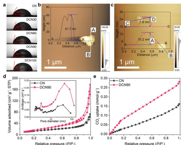
**Fig. 2** (a) Water contact angles of the samples. AFM images and the corresponding height profiles (insets) of (b) CN and (c) DCN90. (d) N<sub>2</sub> adsorption–desorption isotherms, the corresponding pore size distribution curves (inset of (d)), and (e) the CO<sub>2</sub> uptake curves of CN and DCN90.
