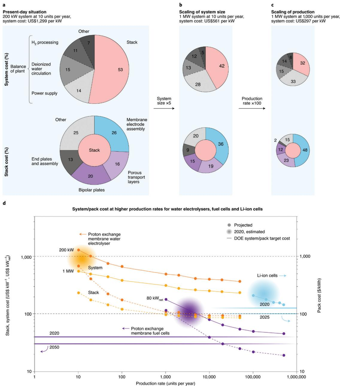
Fig. 21 Cost evaluation of a PEM water electrolyser system. (a–c) Breakdown of system and stack costs for PEM water electrolyzers for the current situation (a), scaled system size (b) and scaled production rate (c). (d) System/pack cost as a function of the production rate for PEM water electrolyzers, fuel cells and Li-ion batteries. Reprinted from ref. 357, Copyright 2020, with permission from Springer Nature.
