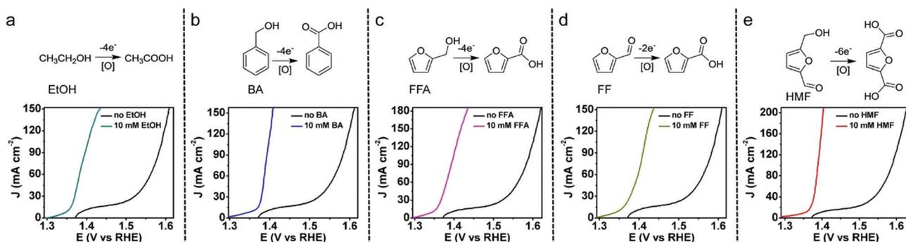
Fig. 16 Polarization curves of the Ni<sub>3</sub>S<sub>2</sub>/Ni foam in 1.0 M KOH for OER and in 1.0 M KOH containing different 10 mM organic substrates including (a) ethanol, (b) benzyl alcohol (BA), (c) furfuryl alcohol (FFA), (d) furfural (FF), and (e) 5-hydroxymethylfurfural (HMF). Reprinted with permission from ref. 300. Copyright 2016 American Chemical Society.
