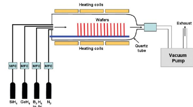
**Fig. 17** Schematic view of the LPCVD system.
