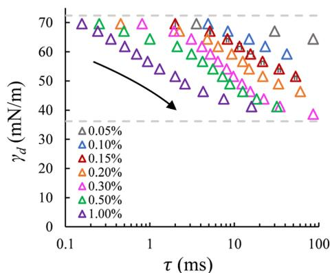
**Fig. 4** Dynamic surface tension versus the adsorption lag time at the a/w interface for a series of SDS concentrations (same as shown in Fig. 3B). Dashed lines: interfacial tension for the bare (upper) and saturated (lower) interfaces with SDS concentrations above  $c_{cmc}$ . Error bars indicate the uncertainty in bubble formation time for repeated recordings (for the data points obtained at 0.15% wt); mostly, the error bars are smaller than the symbols.
