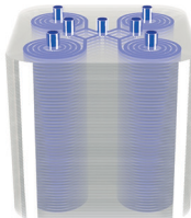
Fig. 1 Development of a mass-producible and deformation-free plastic spiral inertial microfluidic device. (a) A schematic diagram representing the fabrication process of the conventional polydimethylsiloxane (PDMS) spiral device and its stacking process for high-throughput application. (b) A schematic diagram representing the channel deformation in the PDMS spiral device and its effects on the device operation and performance; the color represents the relative channel deformation. (c) A schematic diagram representing the fabrication process of the plastic device and its key advantages; the plastic spiral device was designed by compensating for the channel deformation in the PDMS spiral device.
