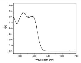
Fig. 3 Solid-state absorption profile for a powdered sample of assynthesised crystals of 1, converted from the experimental diffuse reflectance spectrum using the Kubelka-Munk transformation.
