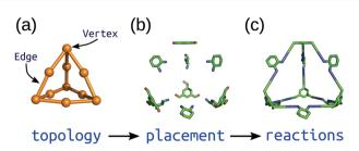
Fig. 4 Schematic of the construction process of an organic cage in stk starting from a (a) topology graph of vertices connected by edges. The supplied building blocks are (b) placed and aligned on the topology, and then (c) "reactions" are performed between them. Reprinted from ref. 95, with the permission of AIP Publishing
